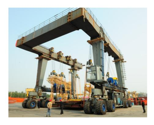
**Mobile Boat Hoist** is used to transfer ship as indispensable lifting equipment by lifting vessel, boats and ship up, then transfer to quay or workshop for repair or storage. They requires a high safety performance and easy operation to adapt local dock design.
